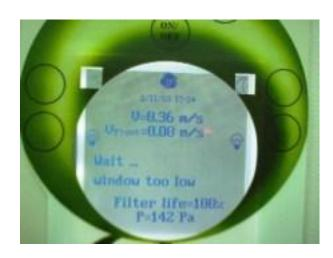
When the cabinet comes back to the normal use, you need to wait until it is displays on the control panel "correct flow" to start to work in the cabinet.
