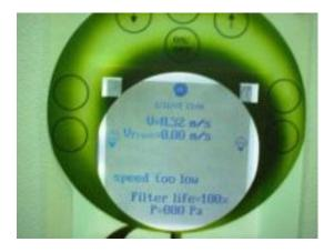
• Window's Alarm: When the window is not in the right position, the alarm beeps and this message appears "Speed too low"
