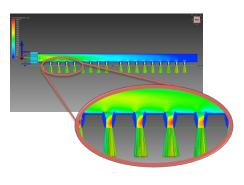
The picture shows how the speed of the fog remains constant despite the variation of pressure along the tube, caused by the distance from the entry point of the tube.
